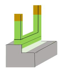
Termicoat® shown in green is not a Termite Blanket System. Termicoat comes with a lifetime treated structural warranty subject to T&C's
