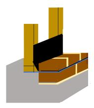
After the TBS is placed and glued the bricklayer returns and places the DPC on top of the TBS and continues bricklaying until the build is complete.
